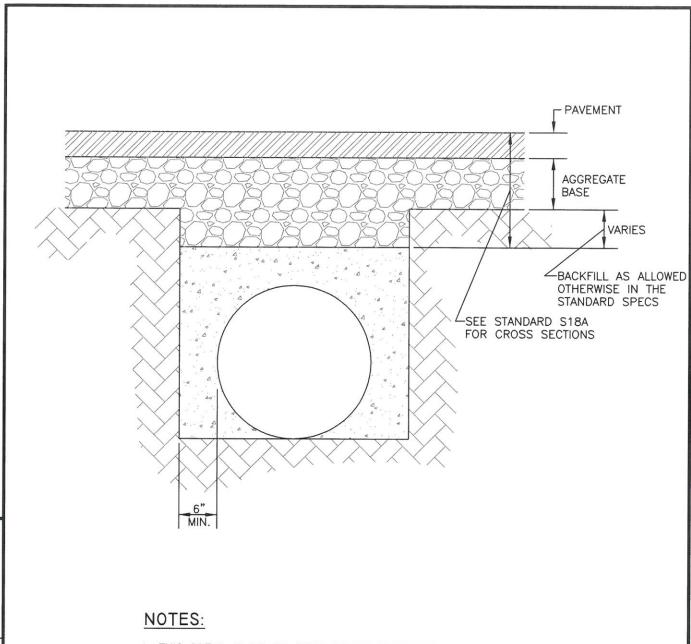
1. THIS DETAIL IS TO BE USED WHERE THERE WILL BE LESS THAN TWO FEET OF COVER BETWEEN THE TOP OF PLASTIC PIPES AND THE FINAL GRADE
