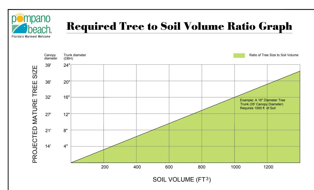
Soil volumes depicted in this chart are based on the amount of roots loam soil can support with optimum compaction for root growth.
