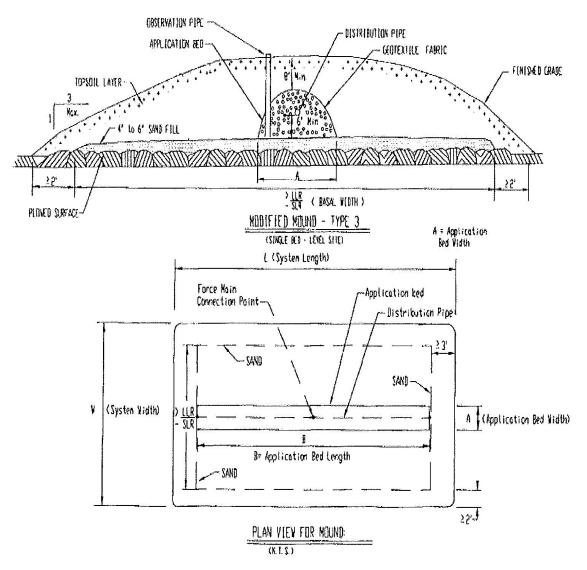
\* Observation pipes may be installed in the application bed.
