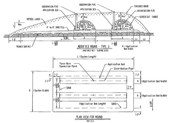
M force noin must connect to the distribution pipe from the upslope or the endstope. The force main cannot be located in the downstope area on landstopes of 2% or greater.
