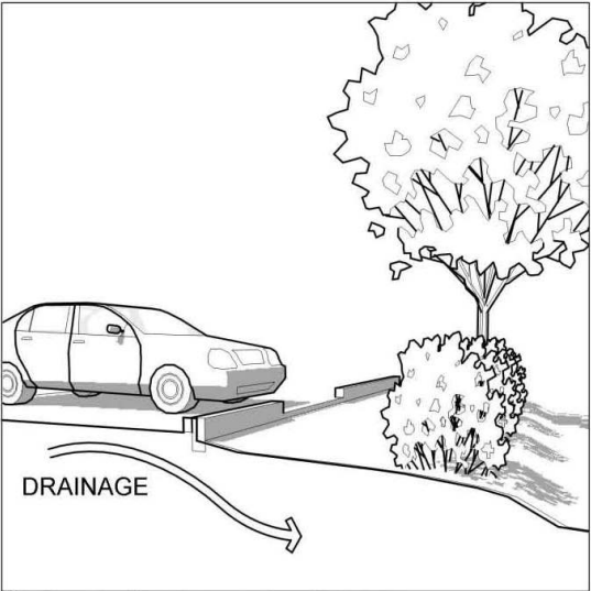
Curb cuts for stormwater drainage
