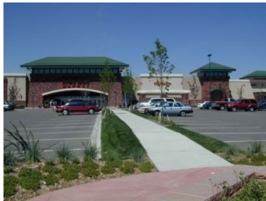
Figure 1234-B: This photograph illustrates how a sidewalk connecting the public sidewalk to the business can be integrated into the required landscaping.
