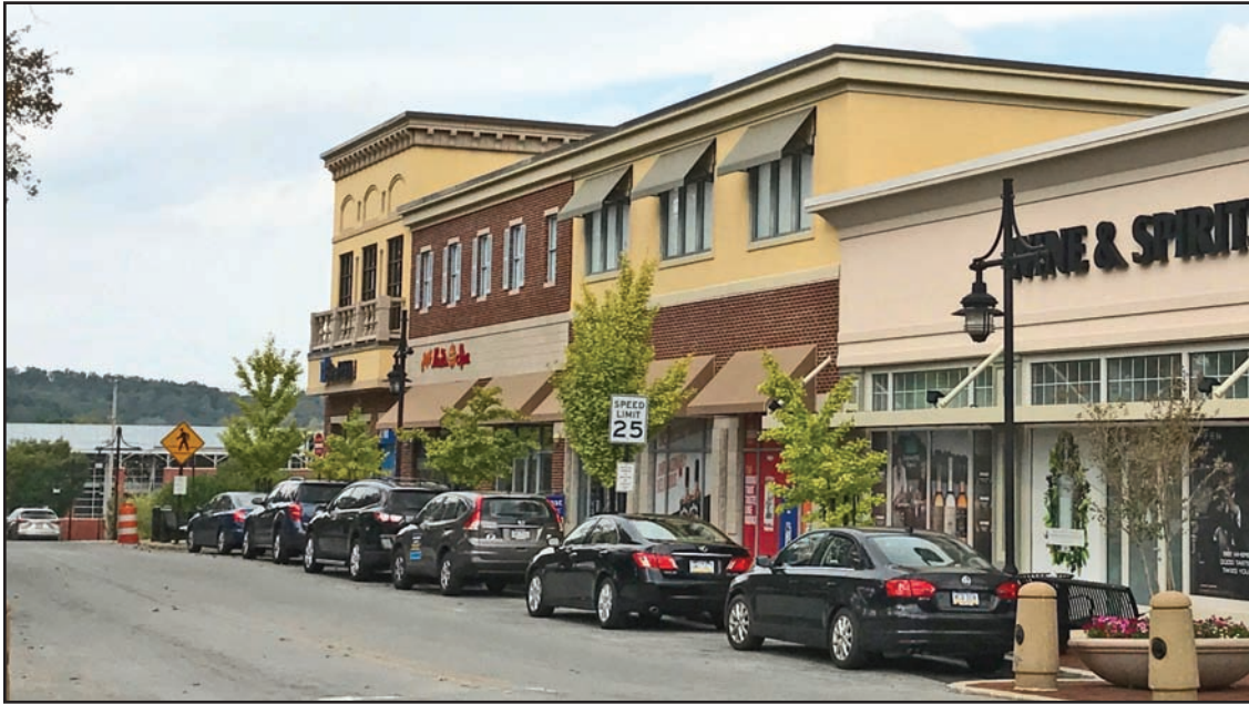
Buildings located at Build-To Line with on-street parking, and a parking lot in the rear
